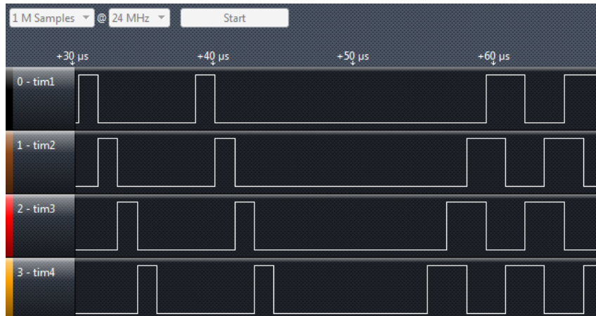
Figure 20: PWM sequence change between 2 arbitrary states
